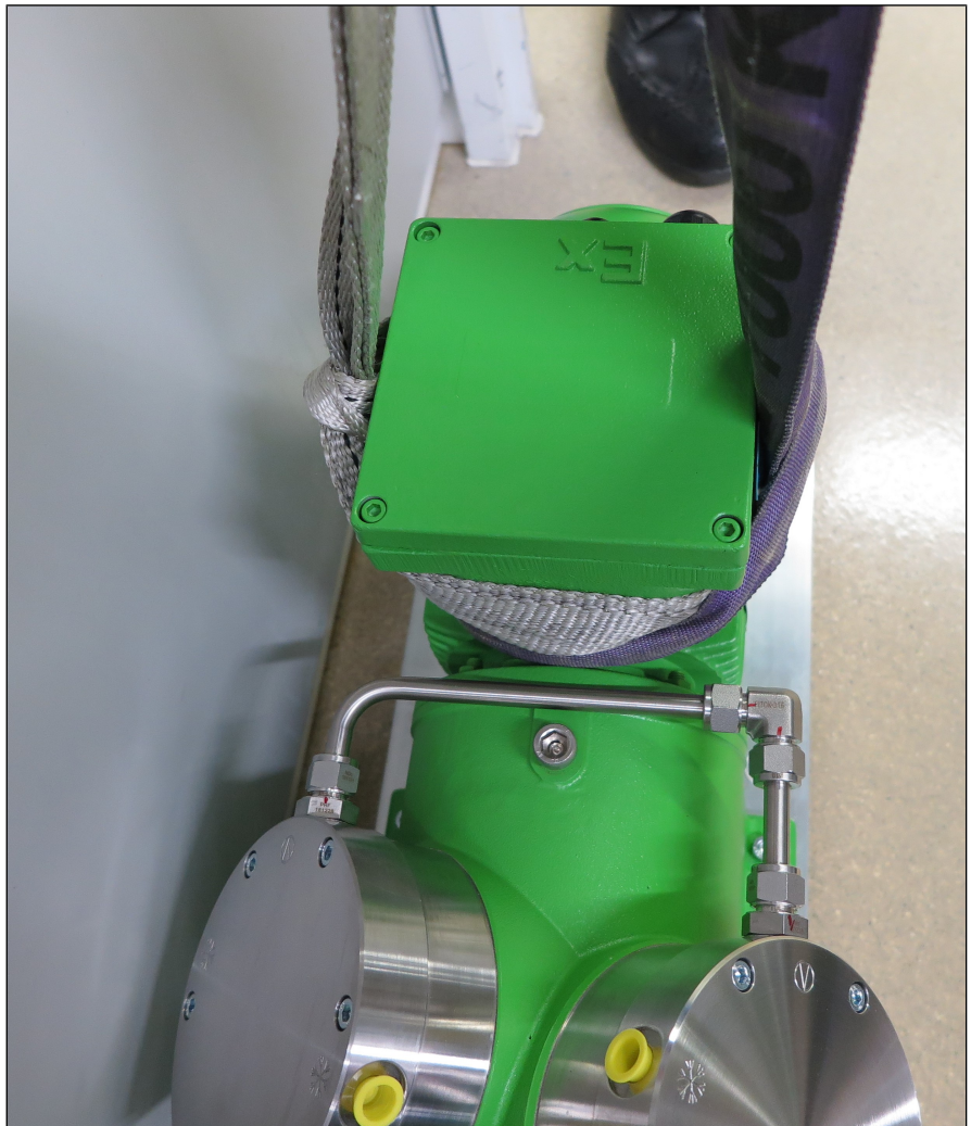
Fig. 17 Lifting motor (depicted pump as an example)
