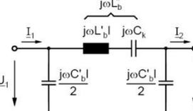
$$j\omega L'_b = j\omega L_b + \frac{1}{j\omega C_k} = j\omega \left( L_b - \frac{1}{\omega^2 C_k} \right)$$
