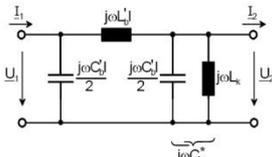
$$j\omega \frac{C'_b}{2} = j\omega \frac{C_b}{2} + \frac{1}{j\omega L_k} = j\omega \left( \frac{C_b}{2} - \frac{1}{\omega^2 L_k} \right)$$
