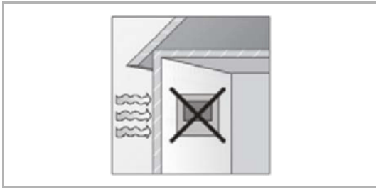
Fig. 5: Installation site - Exterior wall
