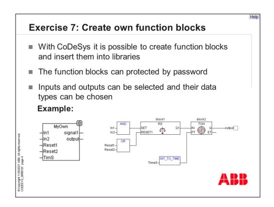
Let's do a little exercise. In the next exercise we build a new function block called "MyOwn". This block includes function blocks and operators from the CoDeSys standard library. The difference between programs and function blocks are that the inputs and outputs must be defined.
