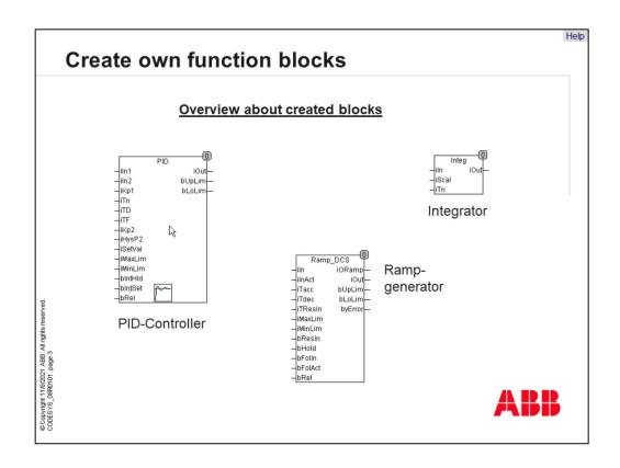
There can be an idea to put several functions into function blocks to hide know how. In CoDeSys it is possible to create own function blocks and put them into libraries. Further the user can define pictures for this blocks, like PID-controller. This function blocks are integrated in a library and can protected with a password. In this case the program code isn't visible for other users.
