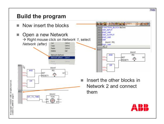
When the new network is designed, we have to put in the several function blocks. If Network 1 is ready, we add a new network after the first one and put in the other blocks. It will be avoided to split the whole program in several networks. So, it is easier to document the networks and get an overview about the whole program.
