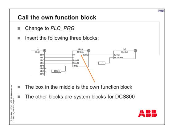
When the new function block called "My Own" is ready we can work with them. So, we change to the POU "PLC\_PRG" and build an application like in the picture. Now the project is ready, and we can test it.
