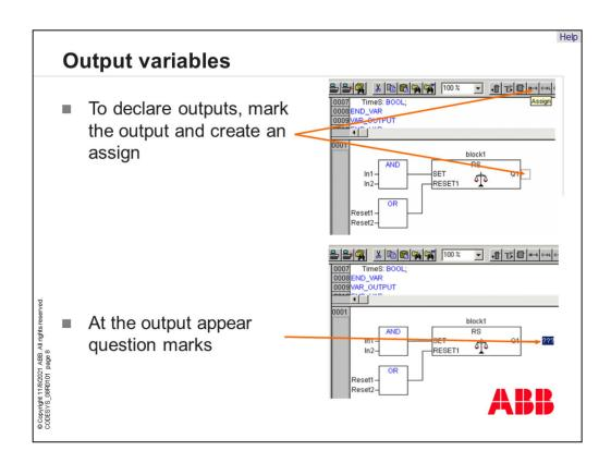
In programming language "Function Block Diagram" the first output at a function block has no connecting point. So we have to add a "Assign" and question marks are shown on the output. Now a variable for the output can be defined.
