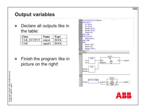
We have 1 output of the new function block. Now this variable must be declared as output variable. The picture on the right side shows the several variables for the function block. We have input variables, output variables and internal variables.
