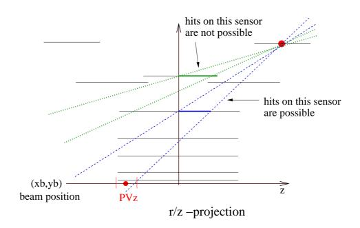
Figure 4.11: Construction of the reference trajectory in rz. The sensor position in z of the  $r\phi$  hit has to be consistent with the primary vertex. The hit has no z information itself but has to be on an intersecting halfladder. With this requirement some arbitrary combinatorics can be removed.
