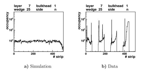
Figure 3.23: The occupancy of the sensor in layer 7, bulkhead 1, wedge 25, side n shows only a partly working sensor in data b). A bit error during transmission transforms the second half of each 128 channel chip to the first 64 channels. All signals seem to be measured by the first half of the chip and the second half seems to have no information. This is not reproduced by the simulation in a).
