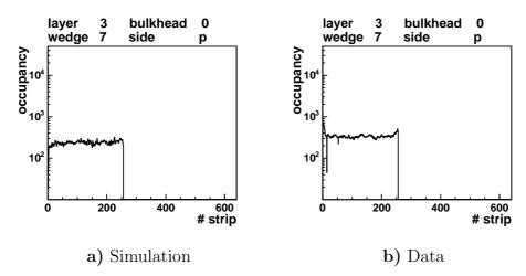
Figure 3.22: The occupancy of the sensor in layer 3, bulkhead 0, wedge 7, side p for simulation a) and data b). The simulation reproduces the same behavior as the data. Only the first two readout chips are working and the other three do not deliver any information.
