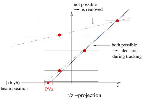
Figure 4.10: Construction of the reference trajectory in rz. The seed track in  $r\phi$  has to be consistent with the z position of the primary vertex.
