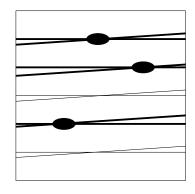
Figure 3.10: Schematic view of the SAS layer. The combination of the strips on both sides results in a clear position.
