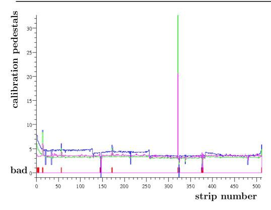
Figure 3.21: The calibration a of sensor in layer 6, bulkhead 2, wedge 16, side p is stored to a database. The bad strips are marked red on the x-axis. The *hot* strips 145 and 325 are identified as bad and a neighbor of a pinhole. The pedestal for these strips is chosen too low and all fluctuations will pass the required charge limit and become a signal. So two very hot strips are the result but these noisy strips are mostly one-strip-hit and can be identified.
