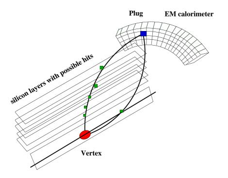
Figure 5.1: Schematic view of the phoenix electron reconstruction. The transverse energy of the plug electromagnetic cluster is used to determine the transverse momentum and the curvature of the electron track. Together with the position of the cluster and the primary vertex a seed helix for an electron and positron can be formed. Along this reference the silicon hits are searched for.
