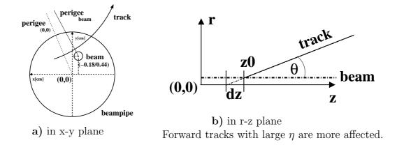
Figure 4.3: Beam offset in data is taken into account by changing the perigee parameters with respect to the beam position.
