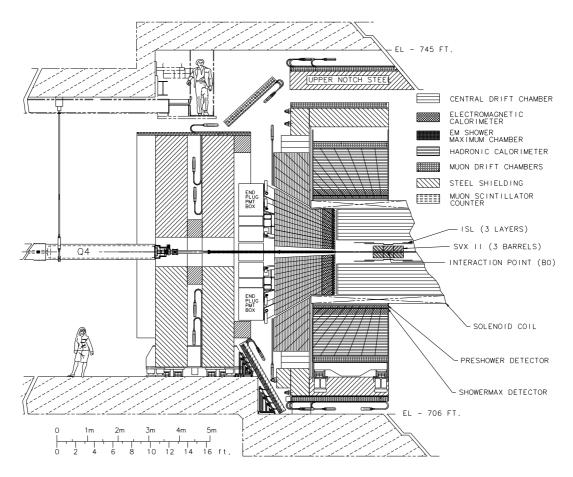
Figure 2.7: Elevation view of one half of the CDF II detector.
