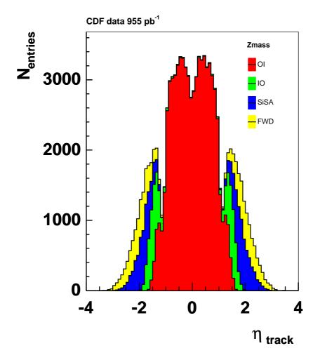
Figure 5.5: The  $\eta$  distribution of the track of the second electron shows the silicon tracks in forward direction. The central electrons are matched with tracks of the OI strategy. The inefficiency at  $|\eta|=1$  is due to the gap between the central and the plug electromagnetic calorimeter. At  $|\eta|=0$ the central electromagnetic calorimeter has some readout electronic devices, which also causes an inefficiency.
