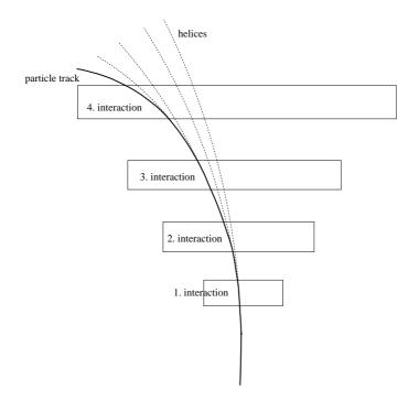
Figure 4.1: An illustration of a particle trajectory with material interactions is shown. The track can not be described by one single helix. Only from one interaction point to the next a helix can be used and so the track is in total a piecewise helix.
