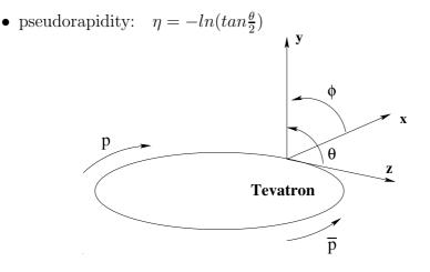
Figure 2.6: Definition of the coordinate system at CDF II.
