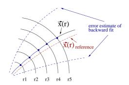
Figure 4.6: The backward fit starts from the outermost measurement and collects information inward. The best parameter estimation is inside the beampipe and is useful for physics analyses.
