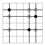
Figure 3.9: Schematic view of the Z90 layer. Three interaction positions result in nine possible combinations.
