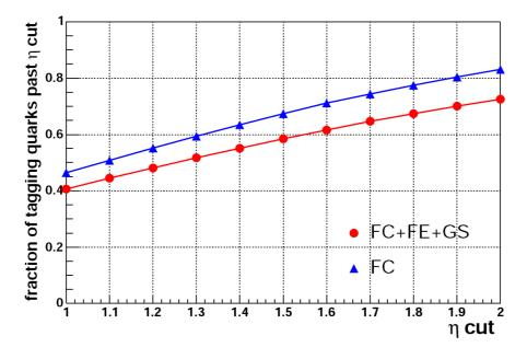
Figure 1.5: Fraction of the simulated  $b\bar{b}$  events with a central *b*-quark and a second *b*-quark passing the  $\eta$  cut on the x-axis. The two graphs are for different simulation models. [3]
