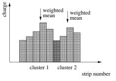
Figure 3.13: Typical shape of clusters with three, two and one strip.
