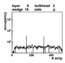
d) Data hits added to tracks : Noise is added statistically to tracks. Hot strips still visible on tracks  $\approx 10$  times higher
