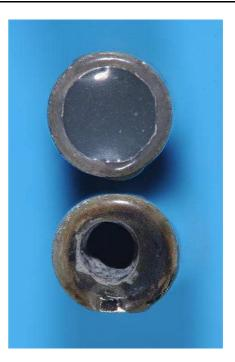
**b)** Cooling line blocked with glue and reopened
