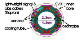
Figure 2.10: Schematic plan view of L00 and the beampipe. L00 consists of 12 wedges on 2 alternate radii with overlapping edges.
