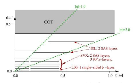
Figure 2.8: Longitudinal view of one quarter of the CDF II tracking system. The layer structure of all three silicon sub-detectors can be seen.
