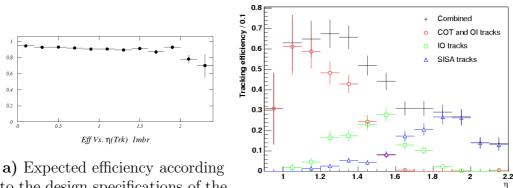
to the design specifications of the silicon detector.
