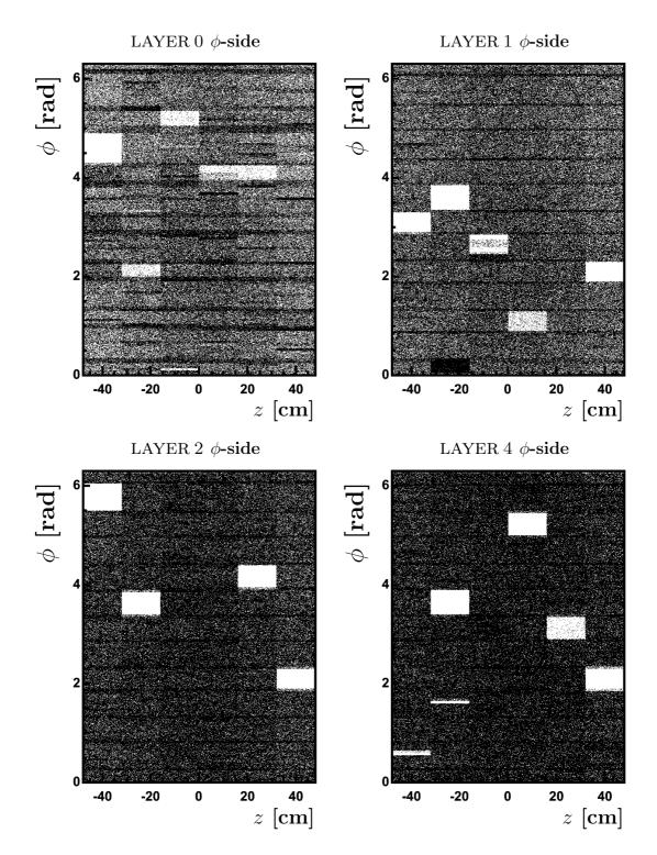
Figure A.5: Map of working  $\phi$  sides in Z90 layers
