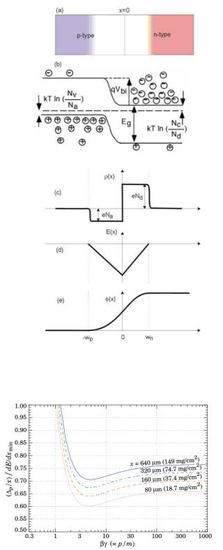
Figure 3.1:pn-junction in thermal equilibrium.a) Schematic view with depletion regionb) Energy band diagram with
