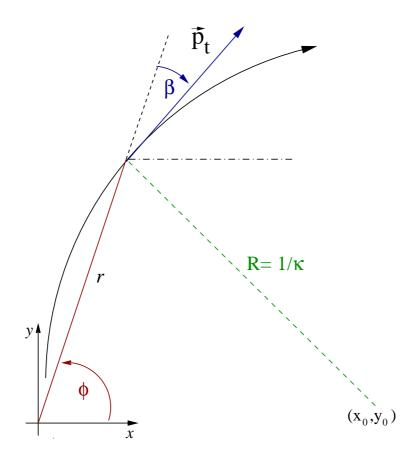
Figure 4.4: Parametrization of a charged particle track in the  $r\phi$  plane. The internal parameters of the TrackingKal package are given at any radii and in local coordinates.
