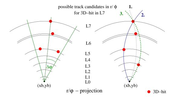
Figure 4.9: Construction of the reference trajectory in  $r\phi$ . All combinations of two 3D-Hits in a small  $\phi$  segment with the beam position are used to construct a seed track for reconstruction.
