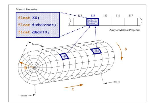
Figure 4.7: The SiliMap is a binned map of the passive material properties. Each map bin holds the index of a description of the average material properties at the position of the bin. Due to the high symmetry of the silicon detector several bins have the same average material properties.
