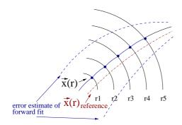
Figure 4.5: The forward fit starts from the innermost measurement and incorporates the information up to the outermost layer. It provides the best parameter estimation outside the silicon and can be used for extrapolation of the track into the outer drift chamber.
