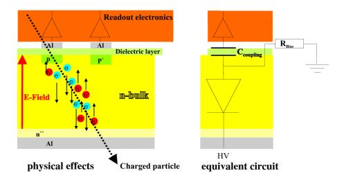
Figure 3.3: Schematic view of a silicon strip sensor. The highly doped p-region is built as strips on the slightly n-doped silicon bulk.
