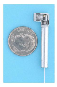
a) ISL cooling line with connection elbow
