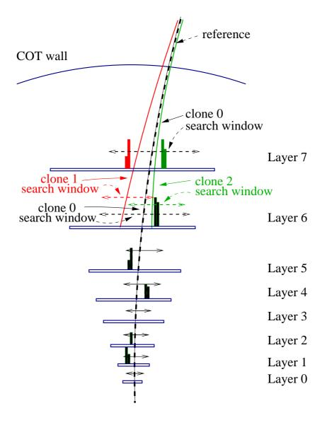
Figure 4.8: A illustration of the hit search along a reference trajectory. For each possible hit, the track is copied, fitted and extrapolated to the next measurement layer. This procedure is continued till the innermost layer is reached.
