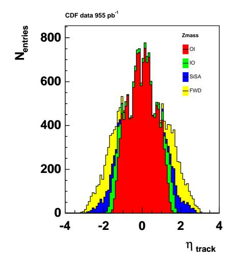
Figure 5.8: The  $\eta$  distribution of the second muon shows the silicon tracks in forward direction. The central range  $|\eta| < 0.6$  has the highest efficiency of muon reconstruction due to the two muon detectors CMP and CMU. The OI tracks at  $|\eta| \approx 1.0$  are matched to the measurements in the CMX. The muons of the silicon track strategies are isolated tracks which can be confirmed by the BMU muon system in the range  $1.0 < |\eta| < 1.5$ .
