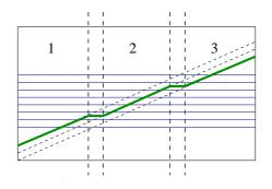
Figure 3.8: Zigzag bonding of the 3 silicon wafers in LAYER 7.
