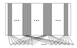
Figure 3.7: Example of the multiplexing of 3 strips in LAYER 2. On the z side three strips are read out via only one channel and so the origin strip of the signal is ambiguous.
