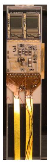
Figure 3.6: In LAYER 1 the 256 strips of the  $\phi$  side are read out via 2 chips located at the outer end of the sensor. This is shown at the top of the picture.
