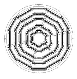
Figure 2.13: Schematic plan view of SVX II. It consists of double sided strip detectors arranged in five layers with twelve wedges each.
