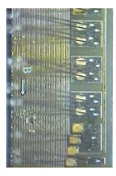
a) Broken micron wires for read out z/stereo sides.
