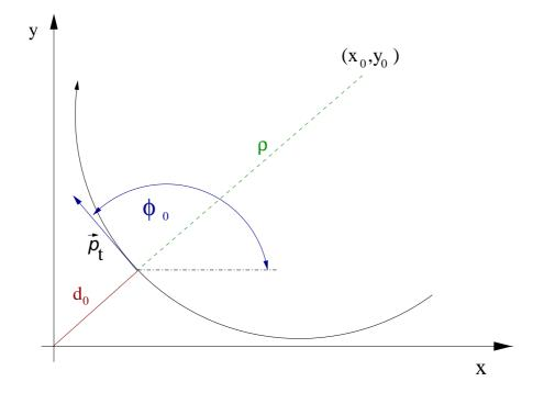
Figure 4.2: Parametrization of a charged particle track in the  $r/\phi$  plane. At CDF II the perigee is used for parameter definition.
