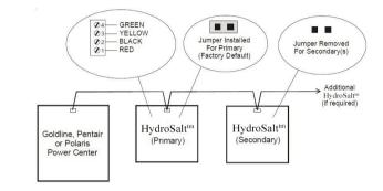
Goldline - Attach wires to proper screw terminals as shown below.
