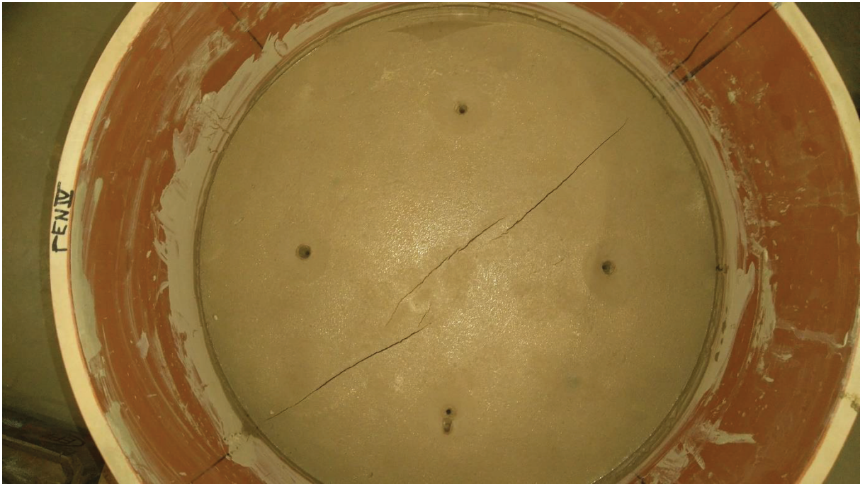
A.M.1 Figure 19 Experimental container with the consolidated and penetrated specimen.
