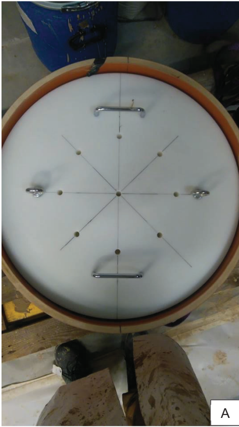
A.M.1 Figure 17 Panel A Top view on the experimental container, showing the pressure plate, which equally distributes the applied pressure from the hydraulic pump. Panel B: Shown here is the consolidation phase of the soil specimen via the hydraulic pump.
