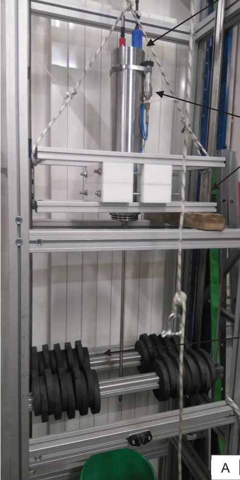
A.M.1 Figure 18 Laboratory free fall calibration tower. Panel A: The laboratory kinematic penetration lance with the pore pressure sensor on its site, built into the free fall slate. The slate ensures the unerring of the laboratory lance. Panel B: The laboratory lance after penetration, slate lays on top of the free fall inceptors
