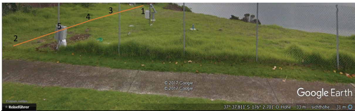
A.M.4.5. Figure 18 Google earth screenshot showing the CPTu transect in relation to the already installed geoscientific observatories such as piezometers at 12 m, 21 m, and 27.5 m, which have been logging continuously since May 2013, as well as waves, wind and rainfall surveillances.
