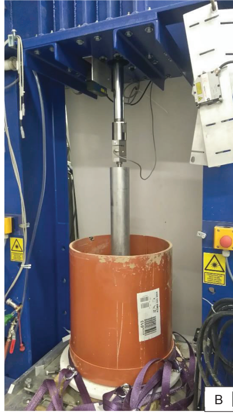
A.M.1 Figure 17 Panel A Top view on the experimental container, showing the pressure plate, which equally distributes the applied pressure from the hydraulic pump. Panel B: Shown here is the consolidation phase of the soil specimen via the hydraulic pump.
