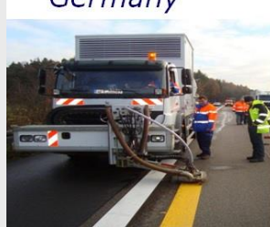
Niederaula, removal Tape/Folie from concrete, 3M Type II 30 cm
