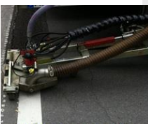
Kumla, removal Thermoplastic Full Line, from soft SMA, 2000 µ – 250 LM/hrs / + Agglo
