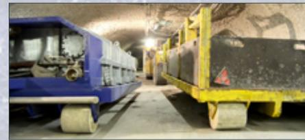
The platforms are designed and manufactured according to customer based specification or application, relevant to the daily operational requirements. After the vehicle has parked, the base unit can be connected to the electrical mains of the mine in the situation that autonomous power supply is required.
