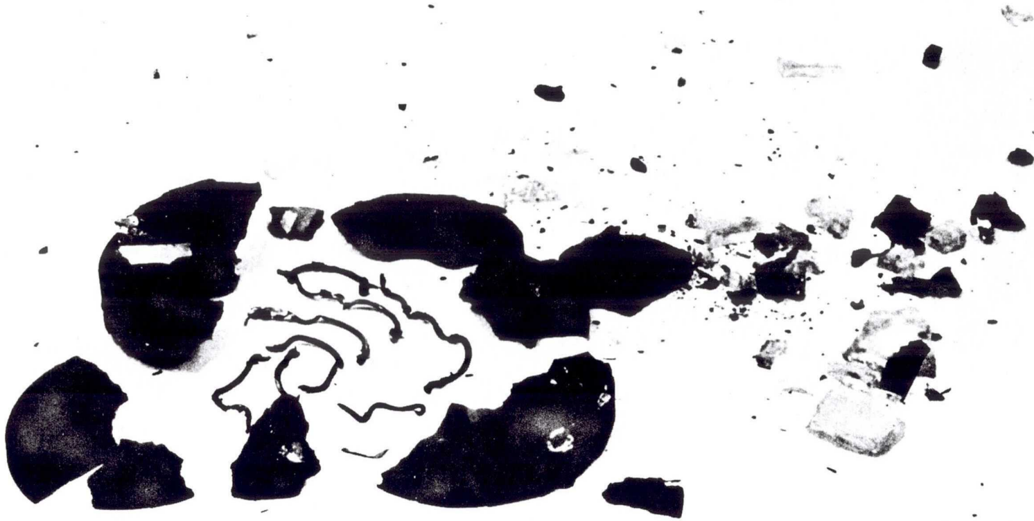
Fig. 31.3 Catastrophic disintegration of test coil by magnetic field.
