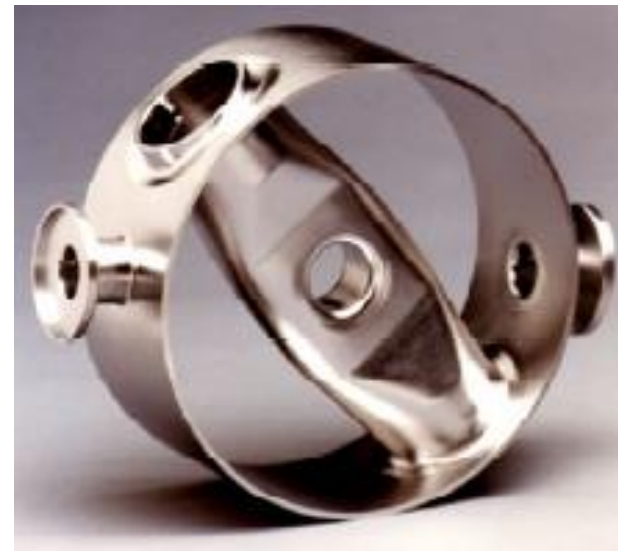
Single Spoke cavity during fabrication
