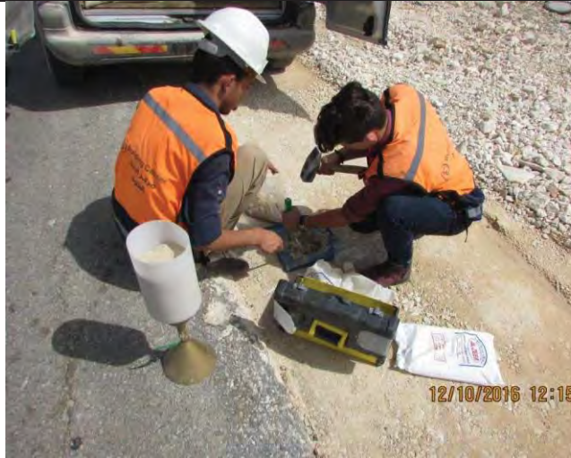
TMN -7 Talfeet – Jalqamous – compaction test for reinstatement works
