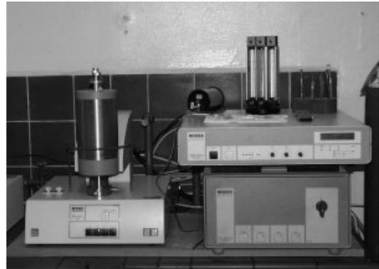
Abb. 2.14: Differential Scanning Calorimetry, ARCS
