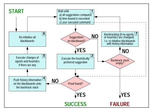
Figure 3.7: The main loop of the automation wrapper.
