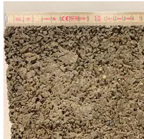
Recycled wooden partikel bonded with cement CEM I 52,5 R (Leube)
