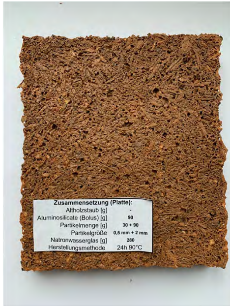
Recycled wooden partikel bonded with sodium silicate
