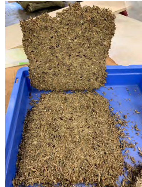
Recycled wooden partikel bonded with urea formaldehyde
