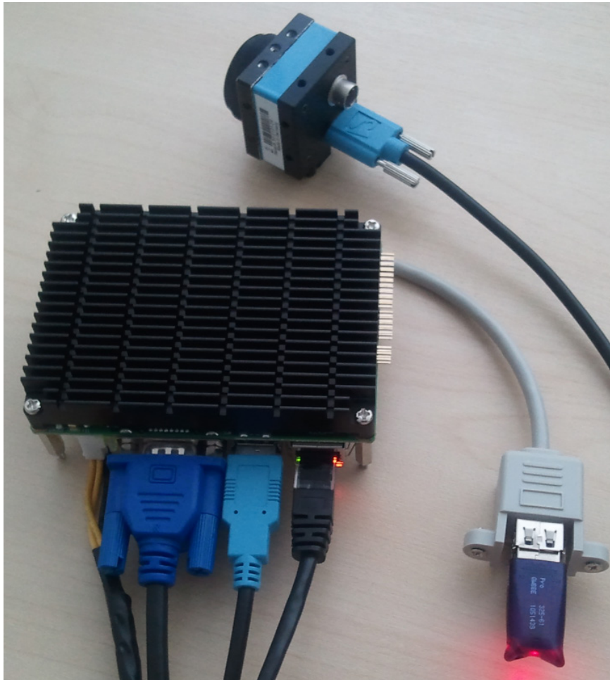
Atom motherboard with a DMK 72BUC02 camera and a VPAR dongle
