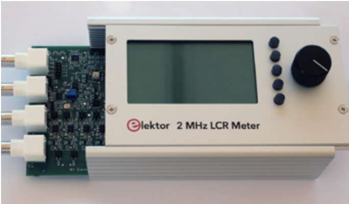
15. Partially assembled LCR-meter during the settings.
