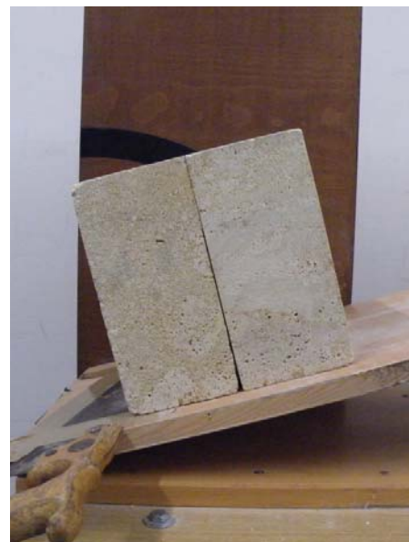
Figure 5: Toppling of two blocks; left: conglomerate; right: sandstone
