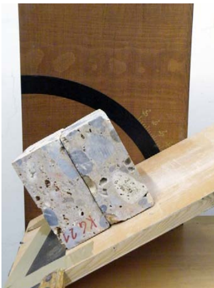
Figure 5: Toppling of two blocks; left: conglomerate; right: sandstone
