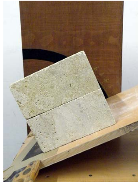
Figure 4: Sliding of a block (tilt test); left: conglomerate; right: sandstone
