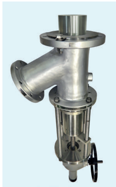
Above: A Type 28KS ram/piston valve with custom replaceable seat, featuring a manual bevel-gear actuator
