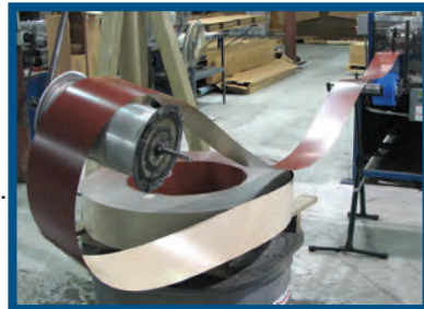
PPC Belden utilizes a proprietary roll form machine to produce exact sizes of cable molding.
