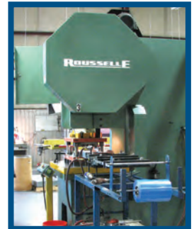
The punch out machine creates custom formed accessories that include corners, tee fitting's and outlet boxes.
