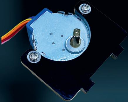
First, place the first, black acrylic frame on your stepper motor and insert the two screws with the two washers through the holes.
