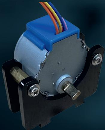
Screw the second, black acrylic frame from the other side with the two screws and washers. Your stepper motor can now be plugged into the receptacle on your Joy-Pi Advanced.
