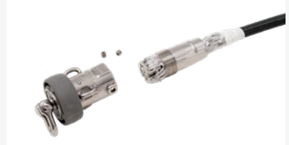
Pull the terminal over the line and fold the core of the line over the wedges. Insert the wedges to the terminal.
