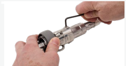
Install the drum/halyard swivel and tighten the locking screw.
