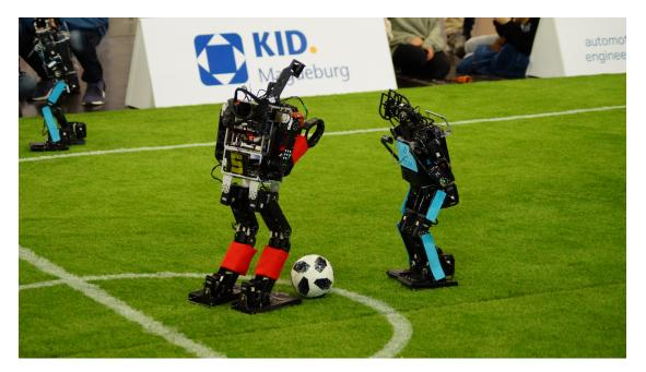
Figure 2.3: Three robots competing in the Humanoid Kid Size League. The Hamburg Bit-Bots in red use their Wolfgang-OP robot while Team Rhoban in blue plays with their SigmaBan robot platform. The differences in regard to e.g. size and proportions can be clearly seen.
