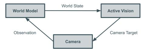
Figure 4.1: This Figure shows the closed loop interaction between the camera, which takes partial observations, the world model which models world dynamics based on them and the active vision component which uses the internal world state to predict a new camera target which closes the loop.
