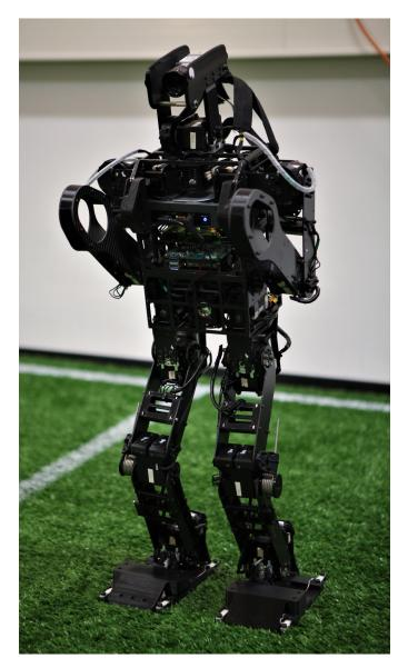
Figure 2.7: A humanoid Wolfgang-OP robot from the Hamburg Bit-Bots. Image used with permission of the owner.
