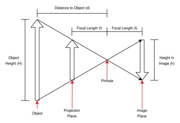
Figure 2.2: Projection of an object onto the projection- and image-plane when following the pinhole camera model. Figure from [Gül19].
