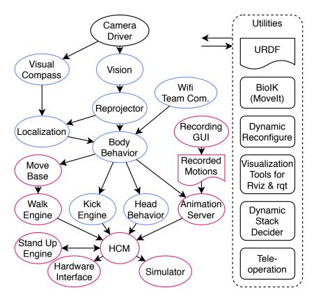
Figure 2.6: Simplified layout of the Hamburg Bit-Bots software stack. Only important nodes and their communication channels are shown. The vision system and the high-level behavior (blue) are specialized for the RoboCup domain, while parts of the motion system (red) are directly usable in other domains. Figure from [Bes+21].
