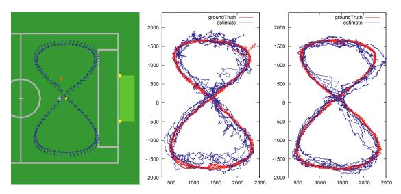
Figure 3.2: Experiment comparing the estimated robot position with both passive (center plot) and active (right plot) camera control. Figure from [SLR10].
