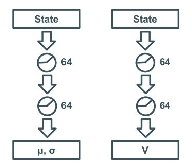
Figure 4.5: This Figure shows the policy and value function networks on the left and right respectively. Both get the same partial observation as an input, which is passed through two hidden layers with 64 neurons each. In the end, the value function outputs the value of the state directly, while the policy predicts both the mean and variance of a multi-dimensional Gaussian distribution that is sampled during training.
