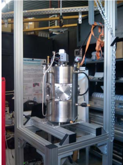
Figure 3.1.: Pressure chamber on the support structure
