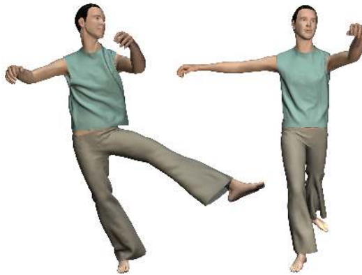
Figure 6: Inextensibility and dynamics. Inextensibility ensures that the tight-fitting pants do not drop past the dancer’s narrow waist. Using fast projection, an implicit treatment of shear and bending, and a mesh with 10600 vertices, the average simulation time per (30Hz) frame was 9 seconds.
