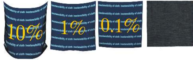
Figure 1: Importance of capturing inextensibility. For efficiency, many simulation methods allow 10% or more strain, whereas many fabrics do not visibly stretch. A 1m 2 patch, pinned at two corners 1m apart, is allowed to relax under gravity. We compare (left to right) three simulations of progressively smaller permissible strain with an actual denim patch.
