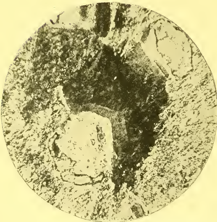
FIG. 19.—Biotite and garnet metacrysts. (See Fig. 20.) 25 diameters.
