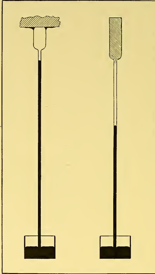
FIG. 2.—Forms of atmometer
