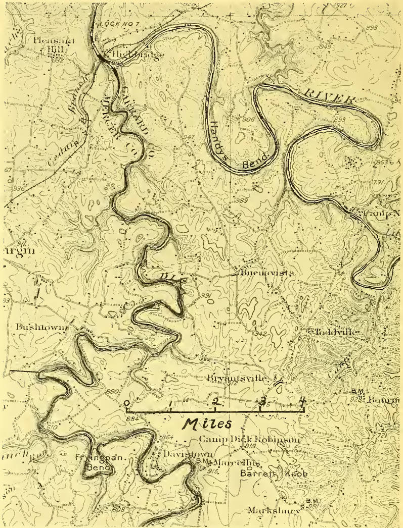
FIG. 2.—Part of Harrodsburg (Ky.) topographic sheet showing typical entrenched meander valleys. Contour interval 50 feet.
