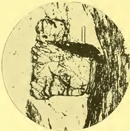
FIG. 11.—Ilmenite bent and inclosed in garnet. (See Fig. 12.) 25 diameters.
