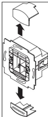
3. Put the protective caps back on the power supply unit.
