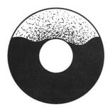
Coarse dirt particles settle on the outer layer depth, whereas finer parts settle on towards the inside increasingly dense layer depth of the **SYNAFELT - Fiber fleece elements**.
