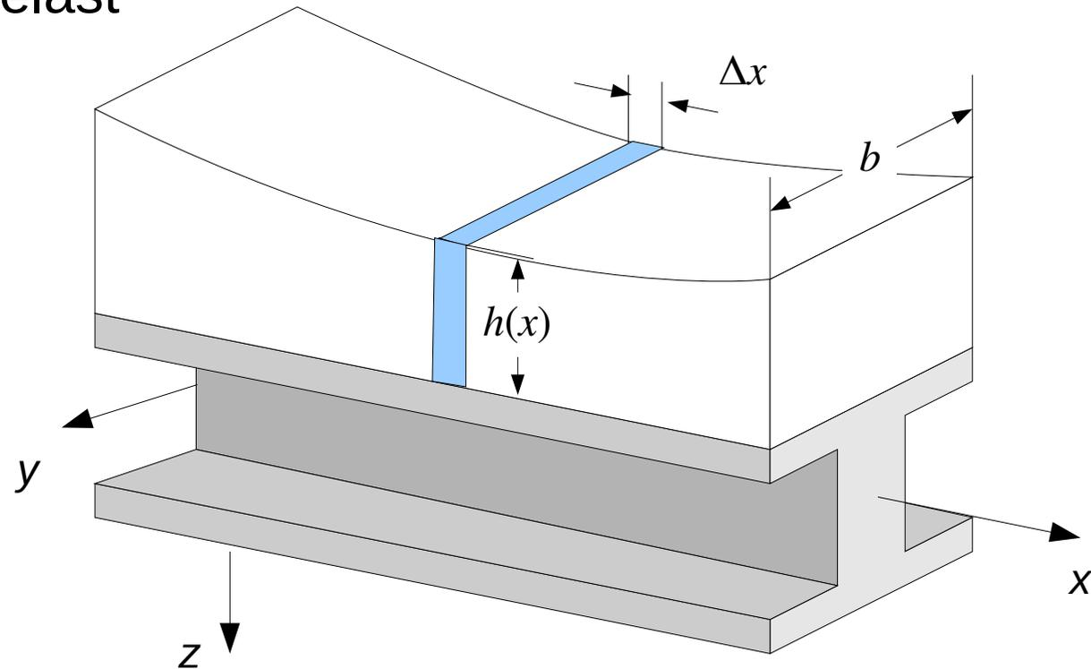
$$\begin{aligned}\Delta G_S &= \rho_S g \Delta V \\ &= \rho_S g b h(x) \Delta x\end{aligned}\quad \rightarrow \quad q_S(x) = \frac{\Delta G_S}{\Delta x} = \rho_S g b h(x)$$
