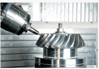
Five-axis CNC milling - max. Ø: 2800 mm
