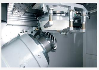
Bevel gear grinding - max. Ø: 900 mm
