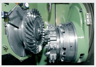
HPG process / hard machining - max. Ø: 1400 mm
