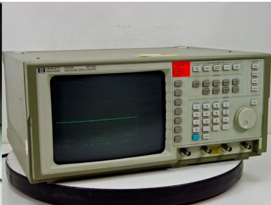
Hewlett Packard 54503A (digital, 2+2 Kanäle, 500 MHz, 20 MSa/s)
