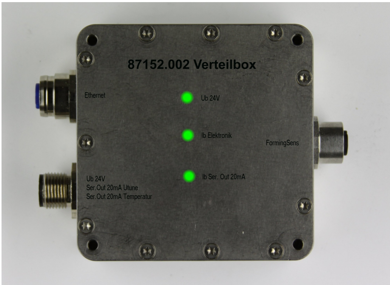
figure 1: connector box with LED indication
