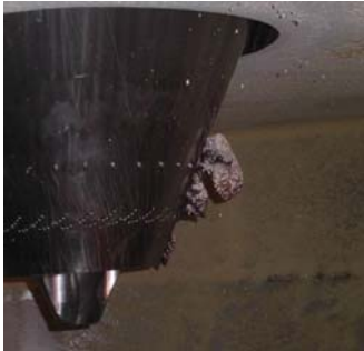
Figure 2: Example of a smoldering dust deposit at the atomizer system
