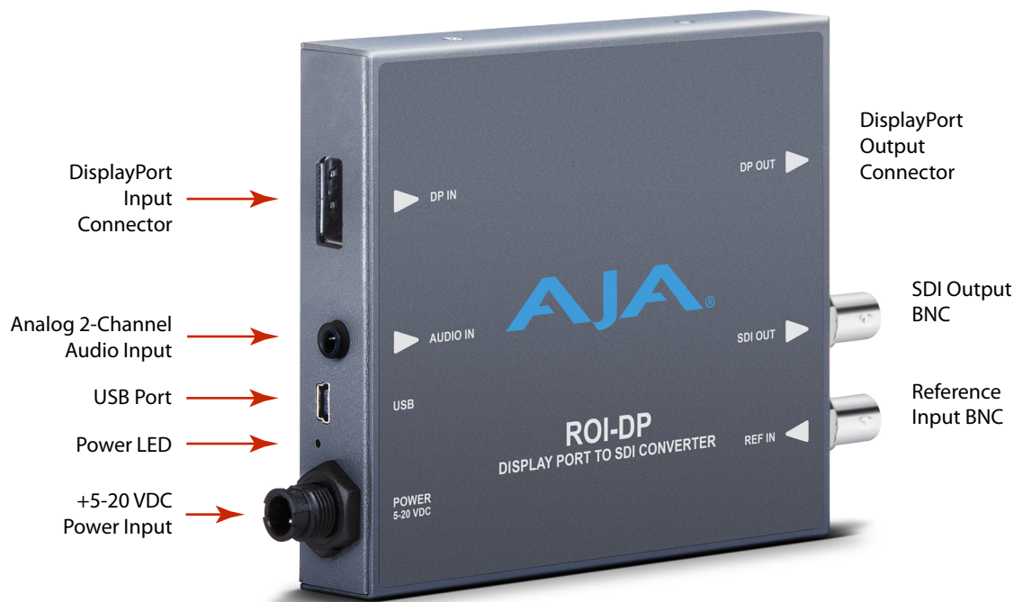
Figure 3. ROI-DP Converter/Scaler
