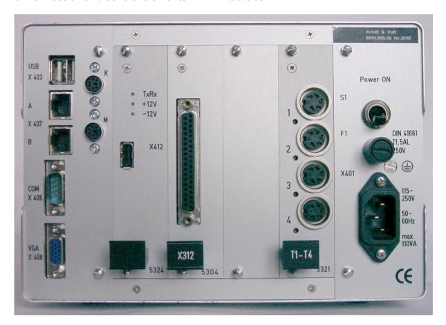
X401 Input power supply 115-230VAC/50Hz
