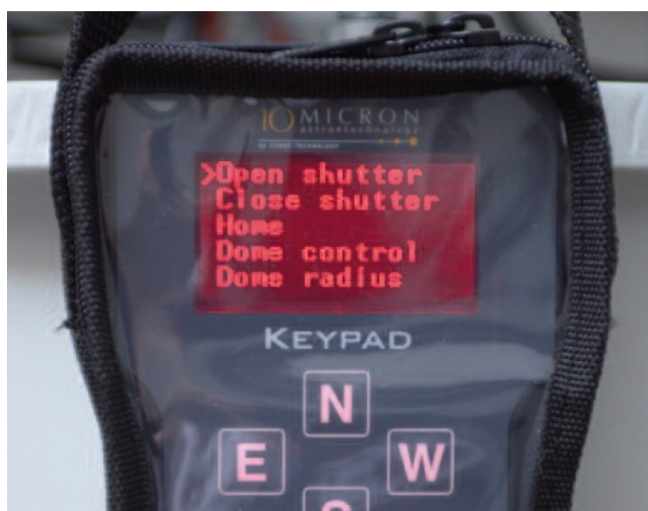
All dome parameters are recorded by the hand box. The whole control is carried out by the clearly arranged menu.
