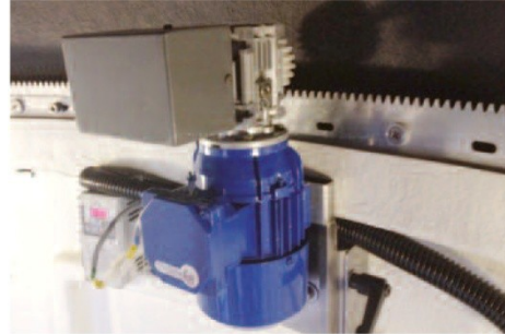
Motor and gear rim subsequently installed by ScopeDome from Poland
