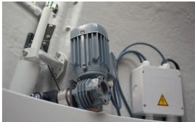
The drive unit for dome gap and dome flap: in case of a total Power failure, manual closing is also possible.
