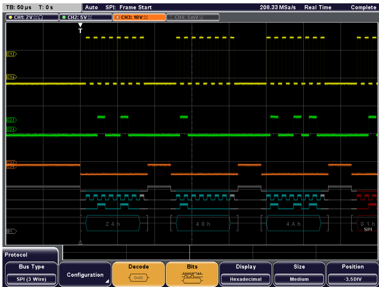
Figure 11-2: Decoded SPI signal
