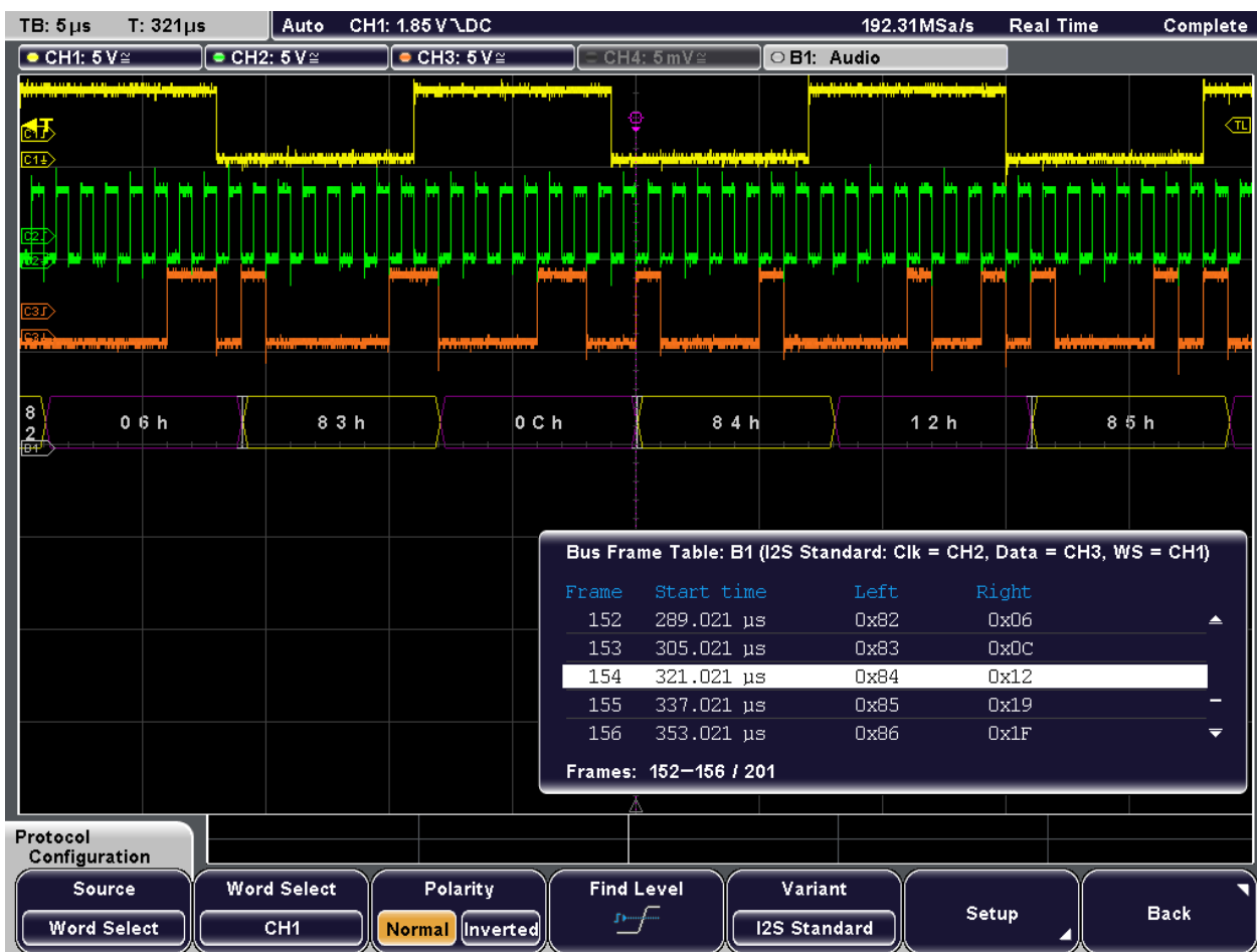
Figure 11-22: Decoded I2S signal with frame table
