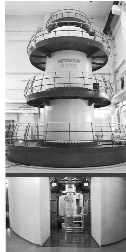
Fig. 1 A general view of the 3 MV ultra-high voltage electron microscope
