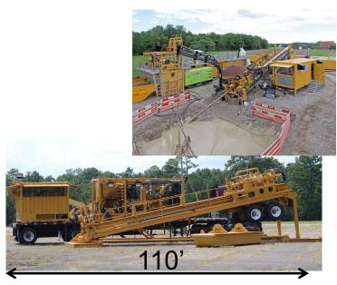
Large HDD Drill Rig >1,000,000 lb Pullback Capacity
