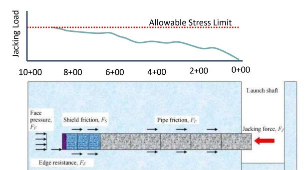
Jacking Force Required (Frictional Resistance Buildup)
