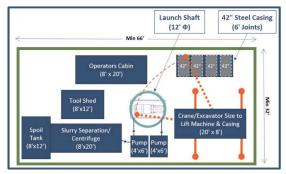
42" Two-Pass MTBM Installation 66' x 32'
