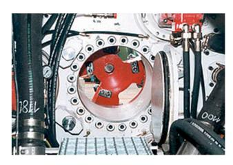
Slurry MTBM with Rock Cutter Head
