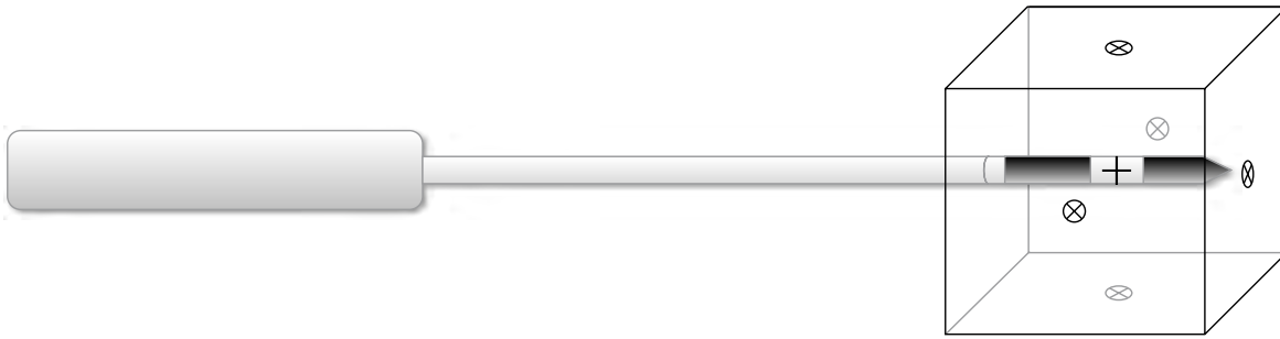
Figure 3: Advanced applicator positioning: While the cross on the applicator marks the initial target position, the center points of the six lateral cube faces are the additional target positions used in the advanced applicator positioning procedure.
