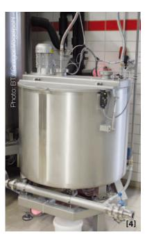
[2] The Dax Dou pre-dough mixer is based on the principle of a continuous flow mixer and is equipped with kneading tools which were developed especially for dough production. [3] Eight silos each are provided for weighing the small components. The ingredients fall through a pipe and directly into the kneading bowl after dosing. [4] After a short mixing phase under ten minutes the liquid yeast is ready to be used and can be pumped into the adjacent storage tank.
