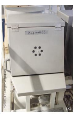
[5] The large external silos with vibration floor are connected to the weighing units via the pipe system. [6] Caraway is a commonly used ingredient in the Frankenland region – and not only for making bread – and is therefore weighed in the small component system.
