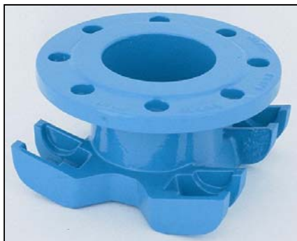
Fig 7.7: Double saddle clamp- drill-clamp with flange pipe size 3" DN 80 PN 4 / 58.0 psig (gas) / PN 16 / 232.1 psig (water)
