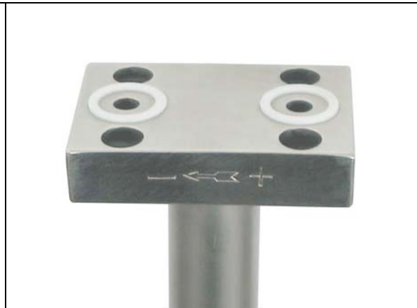
Fig. 7.2: Sensor head with flange plate to direct-mount a 3-way manifold. Limited use w/out pipe insulation, gase to pressure max = 63 bar (914 psig) and temp max = 200 °C (392°F), liquids to pressure max = 63 bar (914 psig) and temp max = 150°C (302°F)
