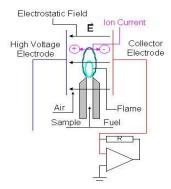
Figure 1. Principle of Flame Ionization Detector Photo courtesy of J.U.M. Engineering
