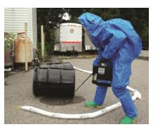
Figure 2. Detecting Leaks from a Chemical Drum Using a Portable FID Photo courtesy of INFICON, Inc.
