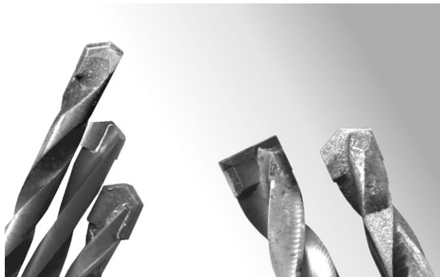
Fig. 3: Five most common drill bits used in drilling resistance measurements. Different tip design (flat or bevelled edges) and substrate material (diamond or Widia-hardened steel) consequently leads to different drilling resistance values.
