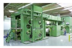
Your orders are processed rapidly and reliably thanks to our modern servodriven printing machines. Due to the sleeve technology, very short set-up times are achieved.
