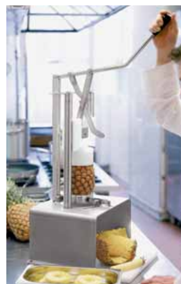
Pela/svuota ananas, inox Pineapple-peeler/corer, stainless steel Ananasschälmaschine, Edelstahl Epluche-ananas, inox Pelador de piña, inox
