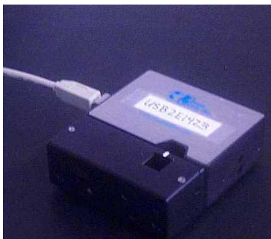
Diode Array Spectrometer with Integrated Visible Source and Sample Compartment
