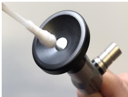
Fig. 4: Cleaning the Proximal Window
