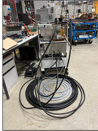
Measurement setup with 20 m cables - for pulse generator protection
