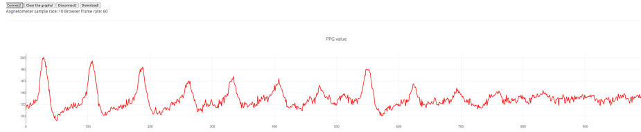
Fig. 5: A web based framework is used to control the BangleJS wristwatch and to capture physiological data from the test participants while they go through the emergency dispatch center scenarios. The above plot shows photoplethysmography (PPG) data with the user’s heartbeats visible as peaks.
